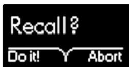
The selected patch is loaded by pressing "Recall" twice. After pressing this key once the display shows "Recall?". If you choose not to load the patch, simply press the key below the word "Abort?" in the display.
